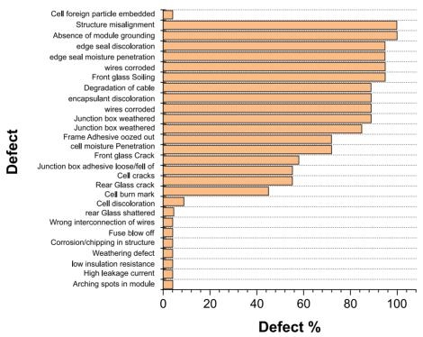
Defects observed in a 2 MW thin film PV power plant
